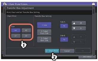
• If you have selected the paper type that cannot be used for auto duplex printing, the message appears and prompts you to load paper manually from the bypass tray. Place paper on the bypass tray and press [OK]. After printing Side A, place the paper with the printed chart Side A face up on the bypass tray and press [OK]. The chart for Side B is printed consecutively.
