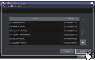
**3** Connect your USB storage device in which the files for updating the system are stored to the USB port on the equipment, and press [OK].
